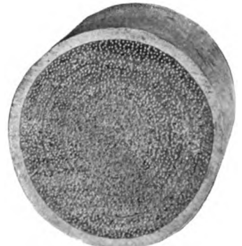
Fig. 48—Cross-section of 1200 Pair Cable
