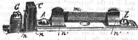
FIG. 7.—Lightning Arrester and Fuse Wire.
