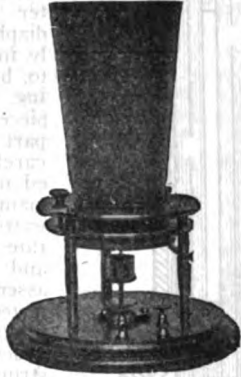
FIG. 5.—The Liquid Transmitter. The first instrument to transmit a complete articulate telephone message.
