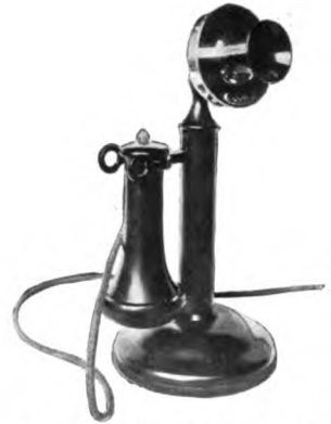
Fig. 29 — Modern Desk Set with automatic switchhook
