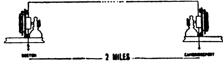
FIG. 7.—Circuit and instruments used by Professor Bell, 9 Oct. 1876. The first time that satisfactory and sustained conversation was carried on by electrical means between persons miles apart.
